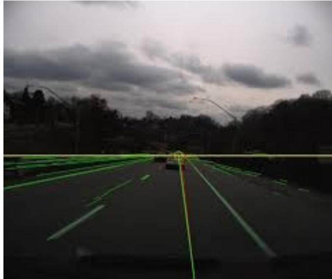
Figure 1: Detection of the vanishing point with lanes and skyline [28]
