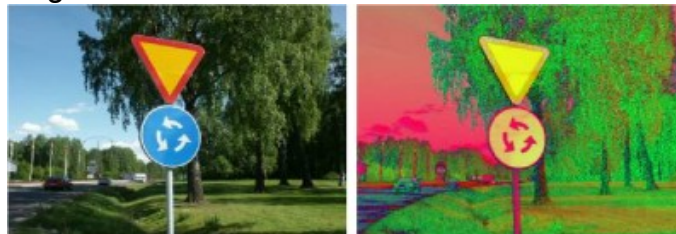
Figure 3: Conversion of an image with traffic sign to HSV color space [26]
